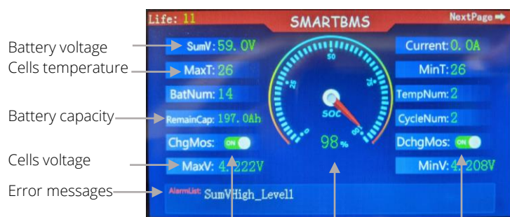
Charge OK State of charge Discharge OK
